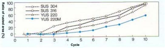
**Test Method:** 10-cycle repetition: Seawater spraying (room temperature) to Drying (60°C×15minutes) to Wetting (50°C, 100% RH×30minutes).
